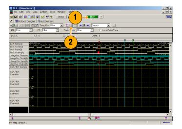
The oscilloscope data appears on the right side of the Waveform window.
