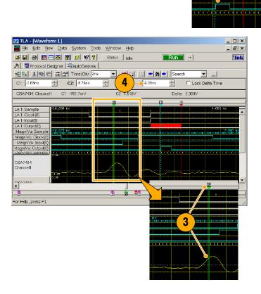
6. Select Time Alignment . . . from the Data menu to open the Time Alignment dialog box.
